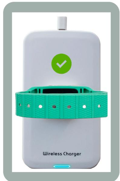
Recharge the mobile device as needed using the charger provided. A routine complete charge cycle is approximately 2 hours. It is best to place the device on the charger with the arm straps connected as shown above.
