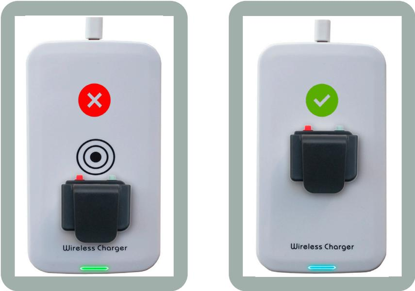
Charging the device while in the beltclip: clip must be face down with belt attachment facing up.
