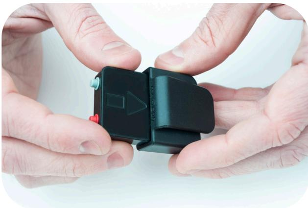
Ensure that the embossed arrow is facing down and toward your body, and therefore is NOT visible when properly placed in the belt clip.
