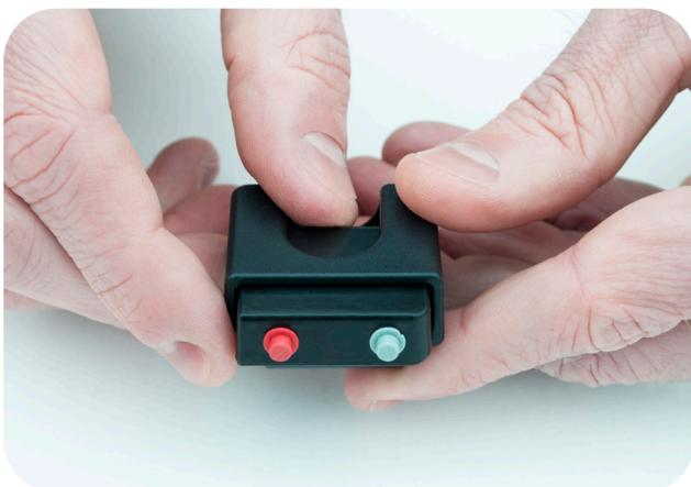
Remove enclosure by using your thumb to push the enclosure upwards and out of the belt clip.
