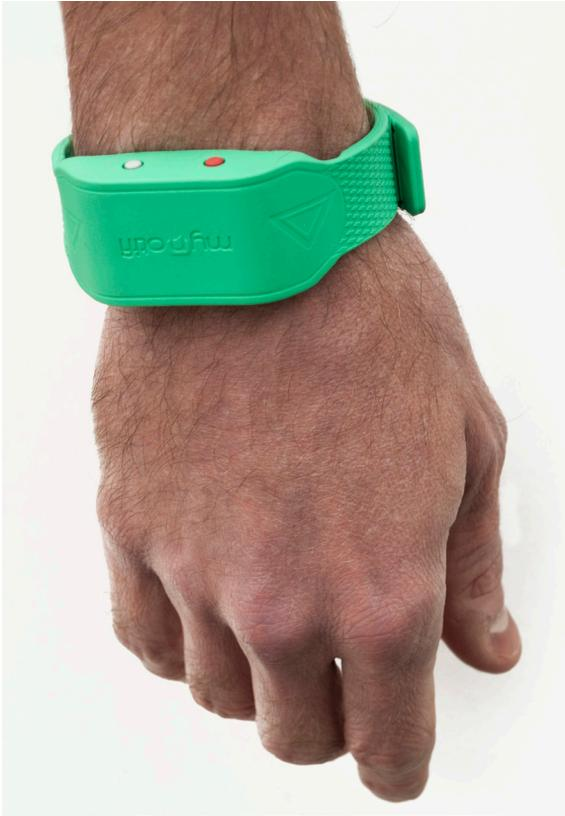
It is also important that the device be worn snug on the wrist and not loose like a bracelet; this will mitigate the potential for false alarms.
